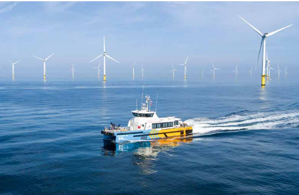
Fig. 2: The Hydrocat 48 with H 2 drive [Source: CMT.Tech]
