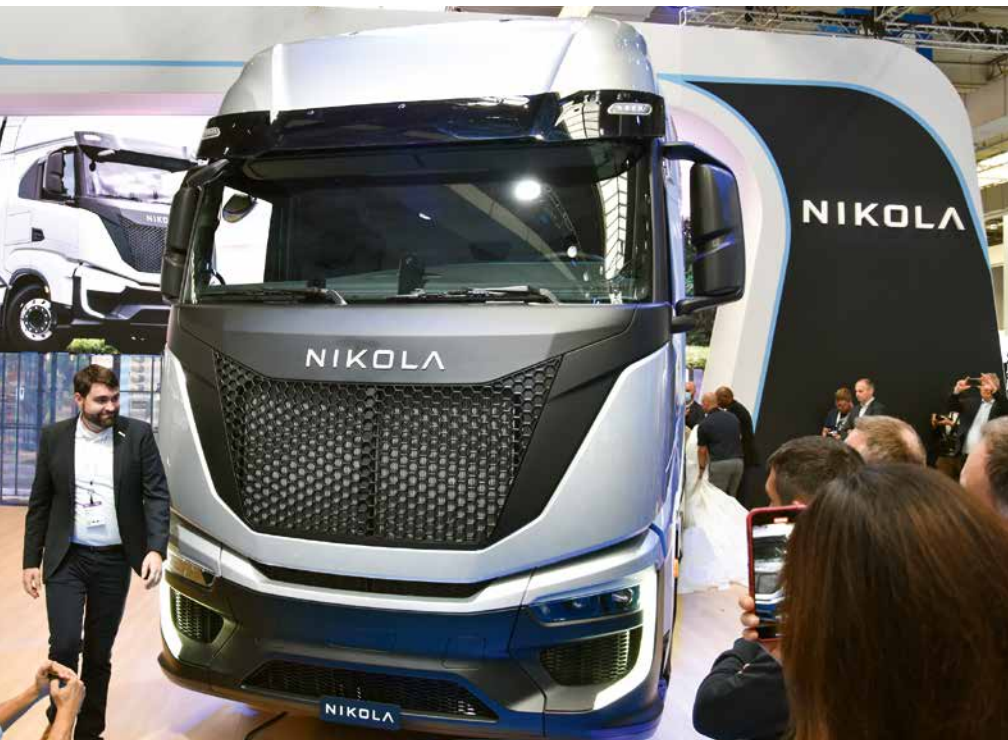
Fig. 1: The Nikola Tre FCEV holds 70 kilograms of hydrogen at 700 bar
