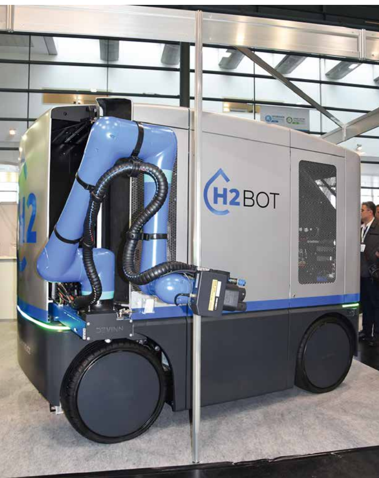
Fig. 1: The H2BOT charges electric cars in situ without the assistance of an operator
