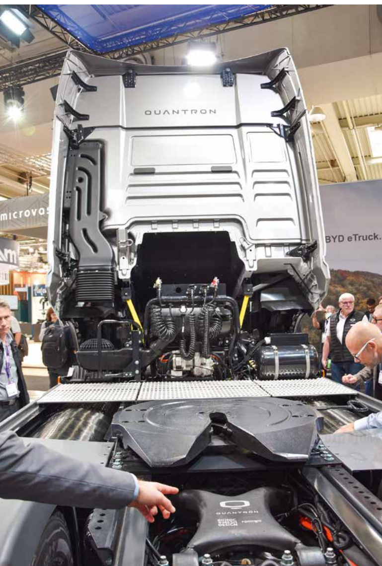
Fig. 4: Quantron truck with Ballard stack inside
