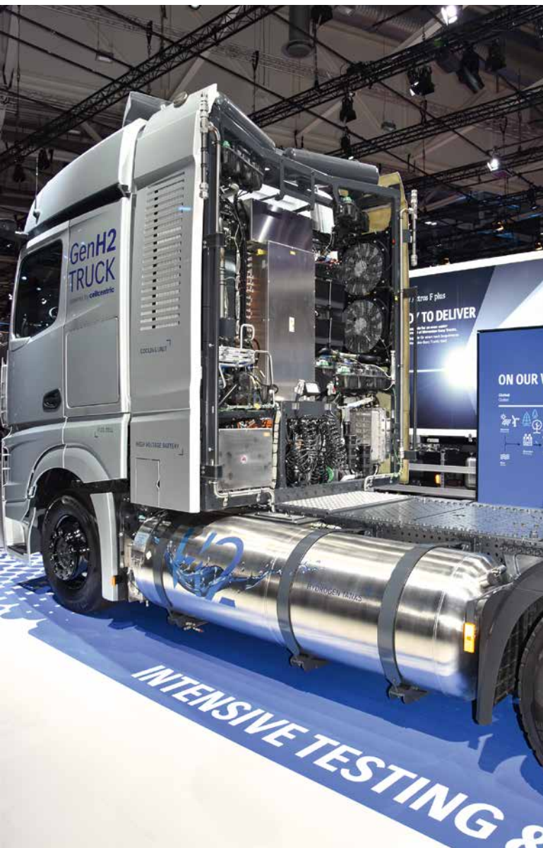
Fig. 6: The two tanks each hold 40 kilograms at -253 °C
