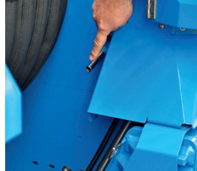
Fig. 3: A thin stainless-steel pipe instead of a wide, dirty exhaust
