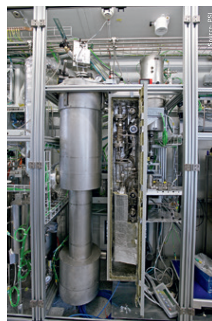
Fig. 4: The fluidized bed reactor, one of four container sections
