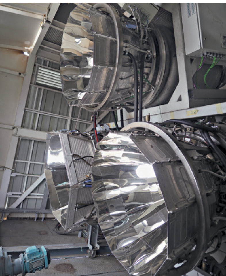
Fig. 1: Front view of the three reaction chambers installed on the solar tower at the Plataforma Solar de Almería
