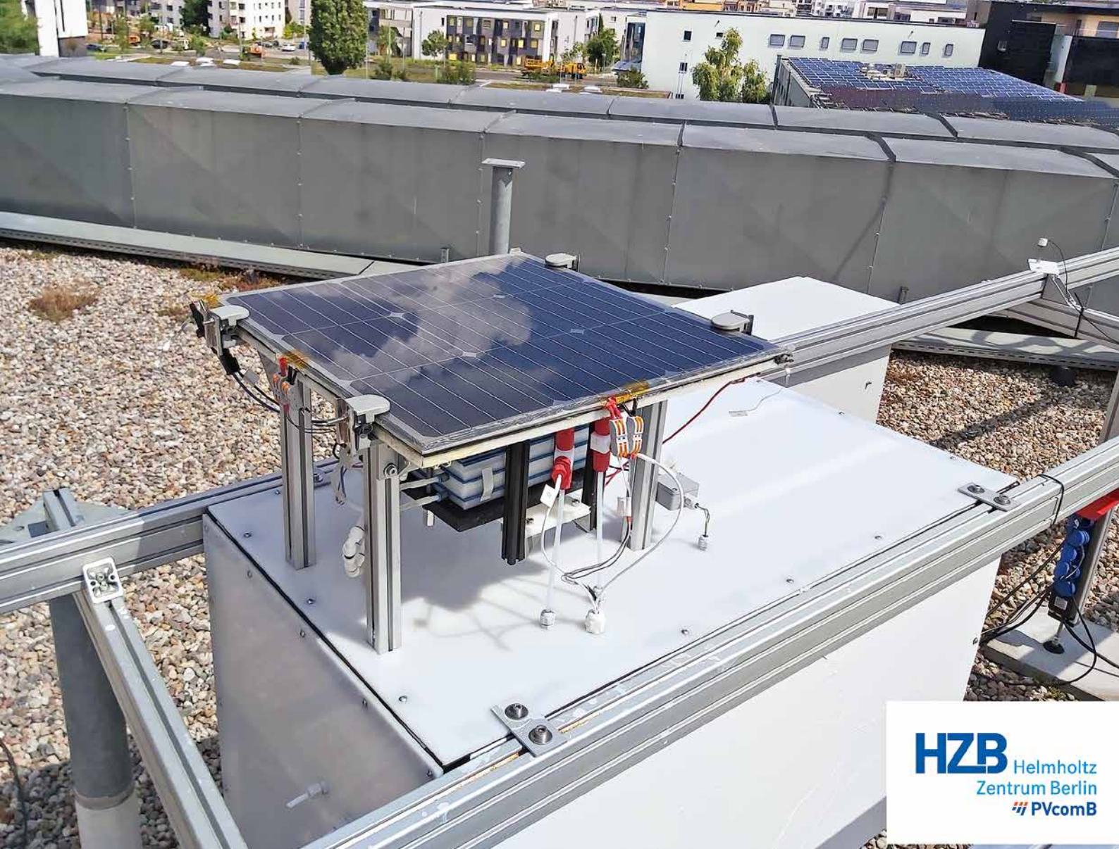
Fig. 1: Above the rooftops of Berlin: The electrolyzers of the test system are the white and blue layers under the PV module.
