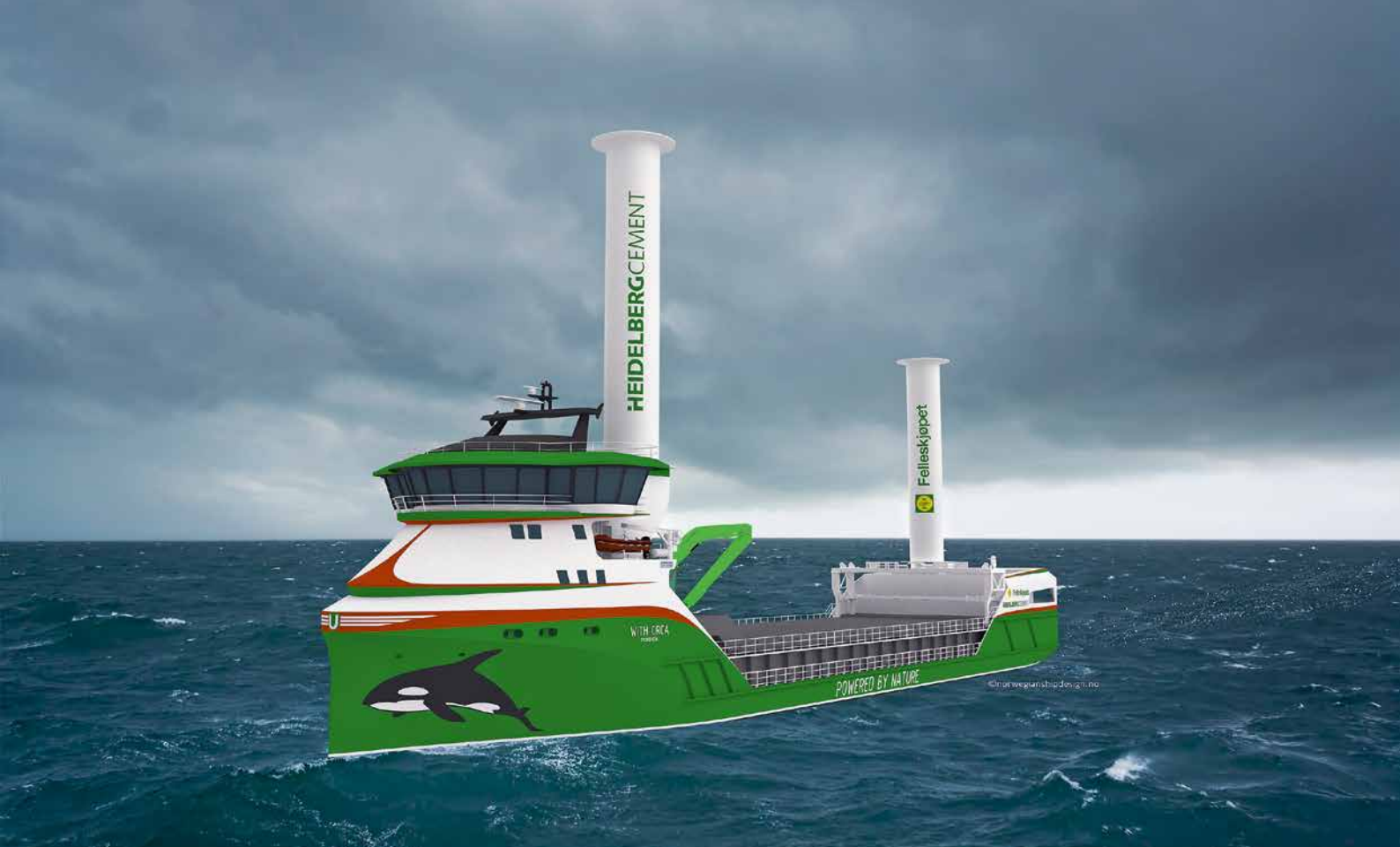
Fig. 2: Hydrogen-powered zero-emission bulk carrier planned by cement maker HeidelbergCement and the Norwegian agricultural supplier Felleskjøpet [Source: Illustration by the partnering companies]
