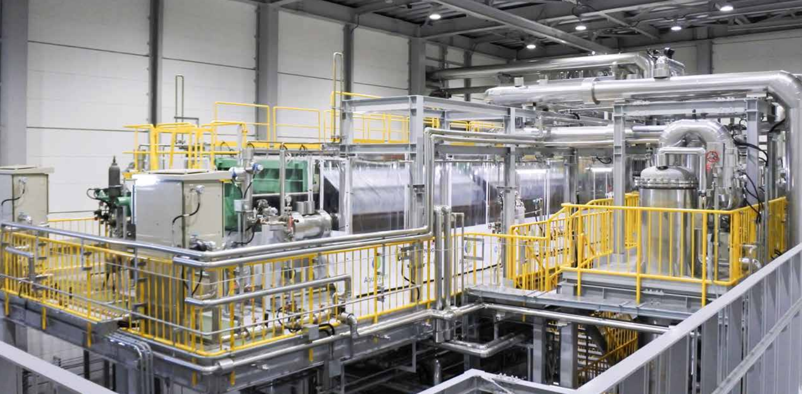
Fig. 3: In March 2020, Asahi Kasei began operating its 10-megawatt alkaline electrolyzer in Namie, Fukushima, Japan – the largest single-stack system in the world [42,000 standard cubic feet or 1,200 standard cubic meters of green hydrogen an hour] [Source: Asahi Kasei]
