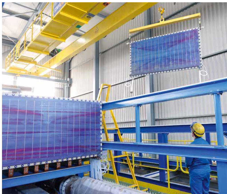
Fig. 4: Modules for alkaline water electrolysis, or AWE, at thyssenkrupp [Source: thyssenkrupp]
