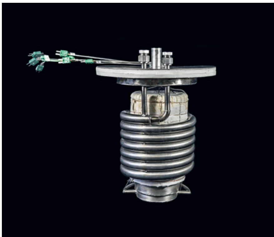
Fig. 3: Ammonia cracker module [Source: ZBT GmbH]
