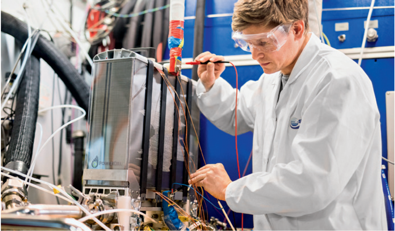
Fig. 3: Testing a 95-kilowatt fuel cell suitable for vehicle integration [Source: ZSW]
