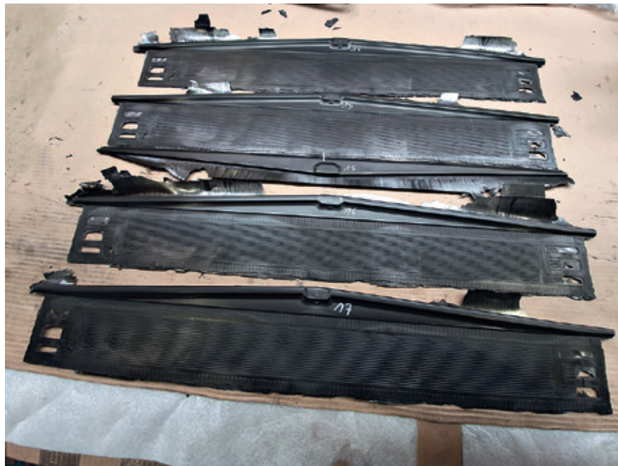
Fig. 1: Large, thin injection-molded bipolar plates [Source: Eisenhuth]
