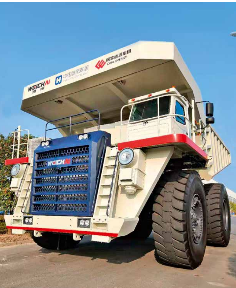
Fig. 1: Weichai mining truck complete with Ballard fuel cell [Source: Ballard]
