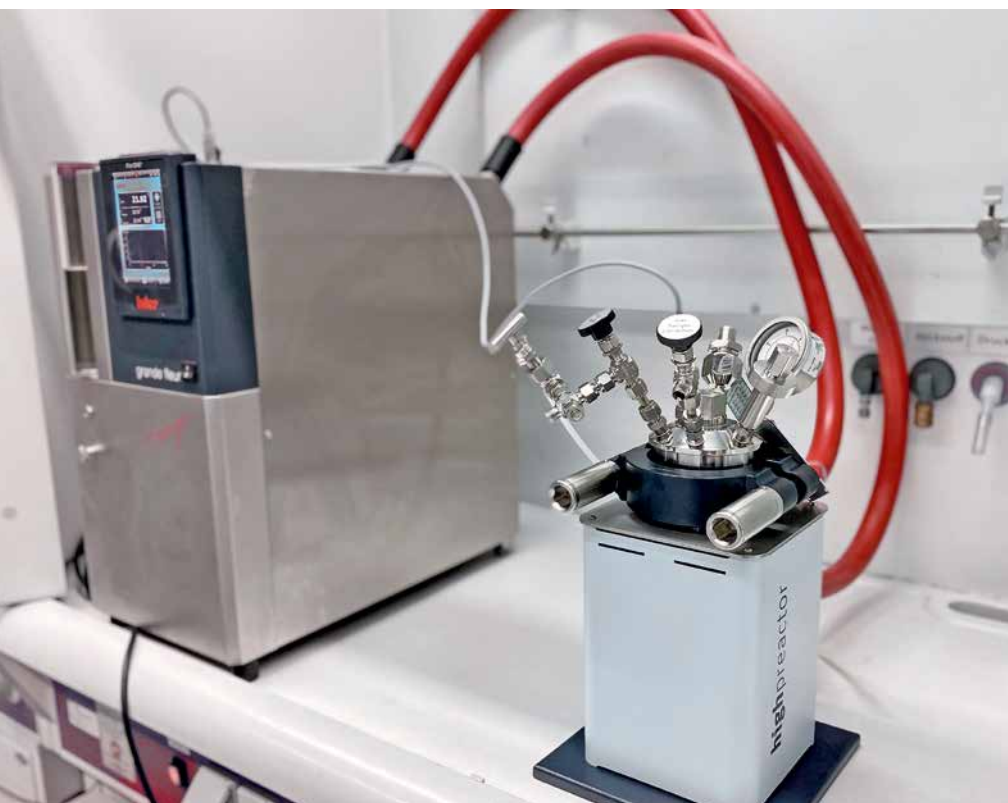
Fig. 3: High-pressure test reactor with temperature control unit [Source: DLR]
